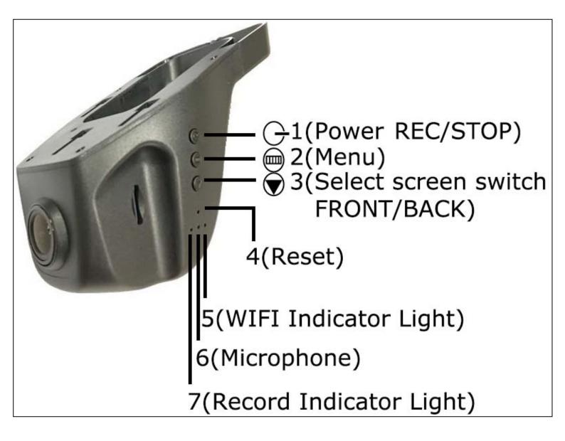
Disconnect the WIFI before using the button operate
